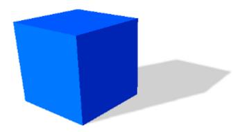
The BoxShape class describes a box collision. The box is aligned with the shape local X, Y and Z axis. In order to create a box shape, you only need to specify the three half extents dimensions of the box in the three X, Y and Z directions.
