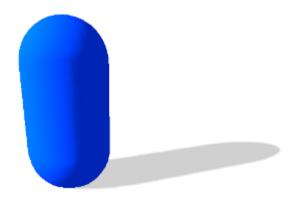
The CapsuleShape class describes a capsule collision shape around the Y axis and centered at the origin of the shape local-space. It is the convex hull of two spheres. It can also be seen as an elongated sphere. In order to create it, you only need to specify the radius of the two spheres and the height of the capsule (distance between the centers of the two spheres).
