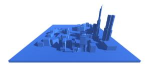
The ConcaveMeshShape class can be used for a static concave triangular mesh. It can be used to describe an environment for instance. Note that it cannot be used with a dynamic body that is allowed to move. Moreover, make sure to use a ConcaveMeshShape only when you are not able to use a convex shape and also try to limit the number of triangles of that mesh because collision detection with ConcaveMeshShape is quite expensive compared to convex shapes.
