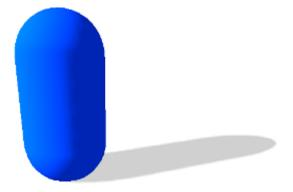
The CapsuleShape class describes a capsule collision shape around the Y axis and centered at the origin of the shape local-space. It is the convex hull of two spheres. It can also be seen as an elongated sphere. In order to create it, you only need to specify the radius of the two spheres and the height of the capsule (distance
